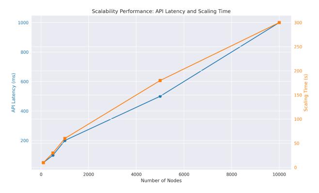
Scalability Performance Description: This dual-axis line graph illustrates how API latency and scaling time change as the number of nodes in a Kubernetes cluster increases.
