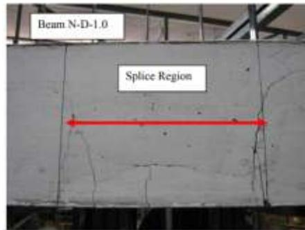
**Fig 1: The fracture pattern of beam N-D-1.0 over the splice region after it failed, as seen from the side face"**
