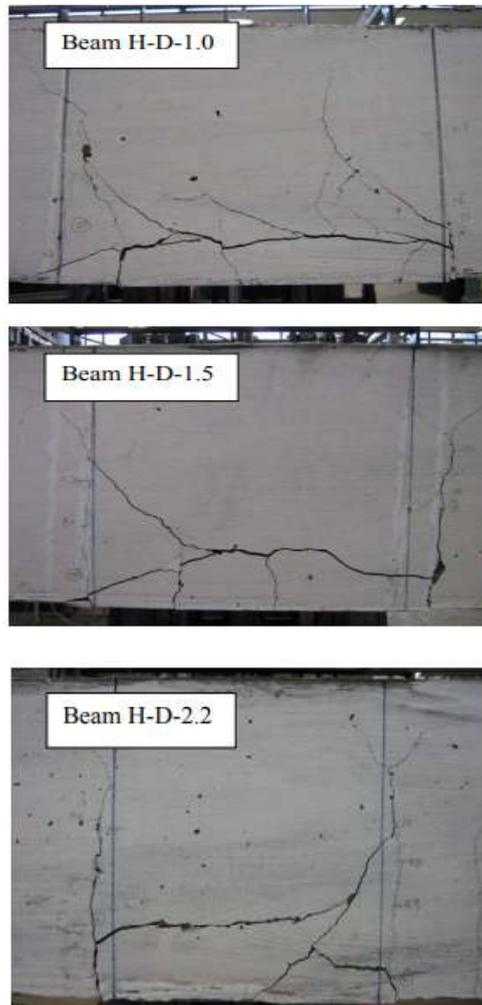
**Fig 5: After failure, crack pattern of high strength geopolymer concrete beams across the splice region (D-Series)**
