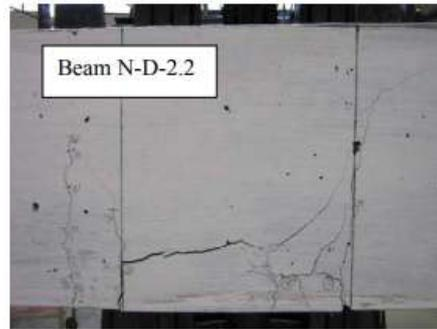
**Fig 4 : The Failure Crack Pattern of Normal Strength Geopolymer Concrete Beams Observed across the Splice Region (D-Series)**
