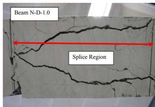
**Fig 2: The failure pattern of Beam N-D-1.0 over the splice region, as seen from the bottom face of the beam**
